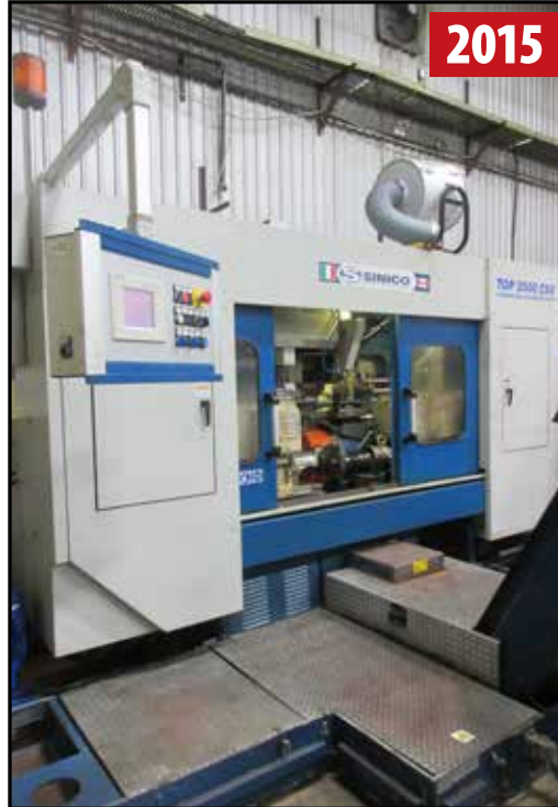
SINICO MOD TOP 2000 TYPE TR 60/4-350 CSV CNC CUTTING/BAR END FINISHING MACHINE
